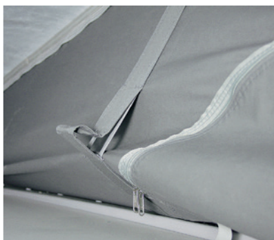
Folding mechanism which pulls the tent fabric inwards in the SCAcomfort and SCAhigh when the roof shell is closed
