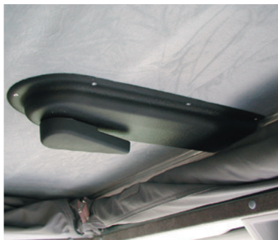
The SCAcomfort's rotary tumbler lock
