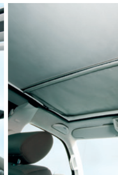
Lined, artificial leather cover, which conceals the folded tent fabric when the roof is closed.
