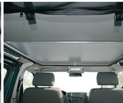
Sliding panel to close access opening in the SCAcomfort
