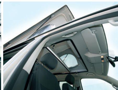
Access to the raised roof bed is through the opening above the front seats. The rolled-up artificial leather cover can be seen in the photo.
